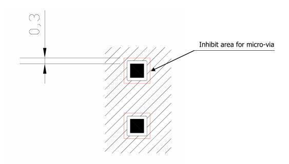
Holes in pad are allowed only for blind holes and not for through holes.
