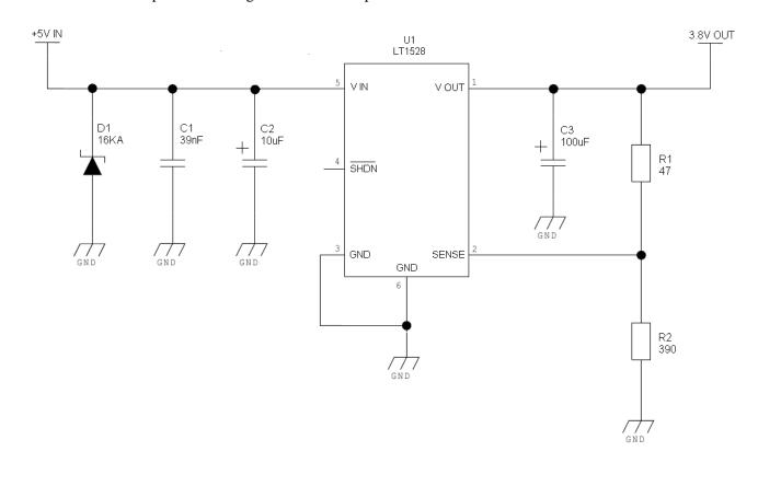
An example of linear regulator with 5V input is:
