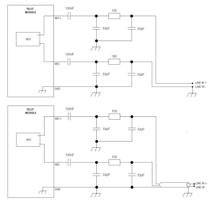
If the audio source is not a mike but a different device, the following connections can be done. Place 100nF capacitor in series with both inputs, so the DC current is blocked. Place the 33pF-100Ohm-33pF RF-filter, in order to prevent some EMI field to get into the high impedance high gain MIC inputs.
