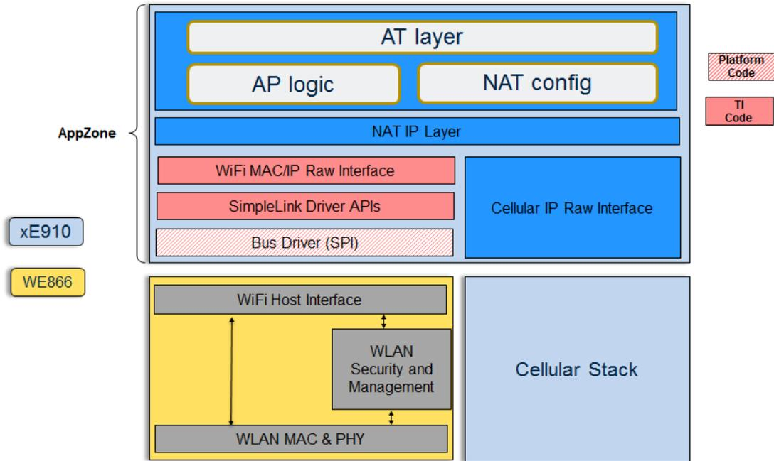
The WE866 is configured in MAC raw mode. All the packet MAC header include will be routed to the cellular module.
