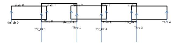
When temperature exceeds the "current state" "threshold", the thermal mitigation algorithm searches the next state when this temperature is lower than "threshold". After it finds it, the "current state" is updated to that "state" and then it checks whether "action" is "mitigate". If yes, then it activates the mitigation according to the "action info" of the "current state".
