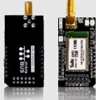
" tRF BoB 70 " is a formative with a microBUS structure. It is an effective and easy solution for adding 868 MHz RF communication to your design. It features the " Telit LE70-868MHz " transceiver module, a SMA connector for an antenna also two radio communication( Tx - Rx ) LEDs. tBoB RF 70 communicates with the target board microcontroller via microBUS UART (Rx, Tx), AN, RST, PWM and INT lines. It has a LED diode in order to power indicator.
