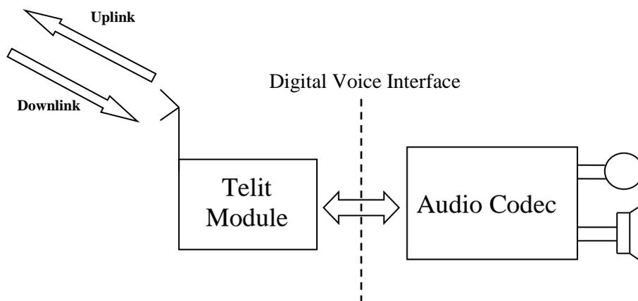
fig. 1: Example of Digital Voice Interface Use
