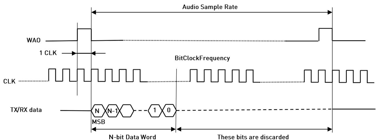
fig. 7: Module is Slave/Burst mode/N bits per sample/Mono Mode
