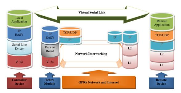
This particular implementation allows to the devices interfacing to the Telit GL865-DUAL/QUAD module the use of the GPRS and Internet packet service without the need to have an internal TCP/IP stack since this function is embedded in the module.
