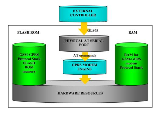
In order to not use any external controller, and further simplify the programming of the sequence of operations, the customer can benefit of these feature already embedded in the GL865:
