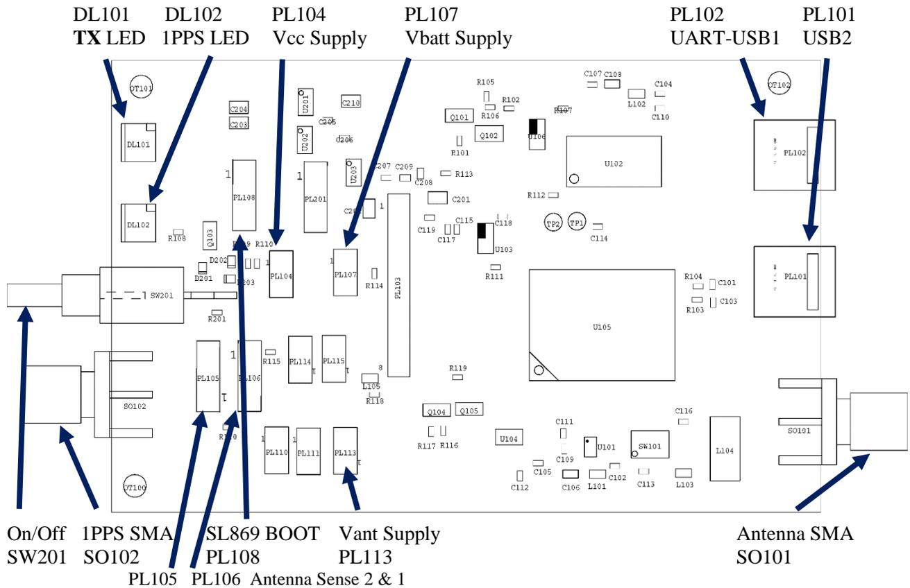
Note: PL105 and PL106 must be jumpered 1-2 to operate the on-board Teseo 3 Antenna Sense circuit.
