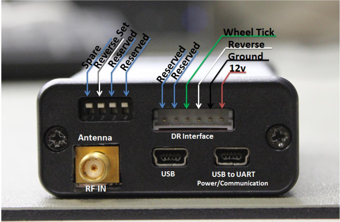
Figure 4-7 EVK Unit connections – rear panel
