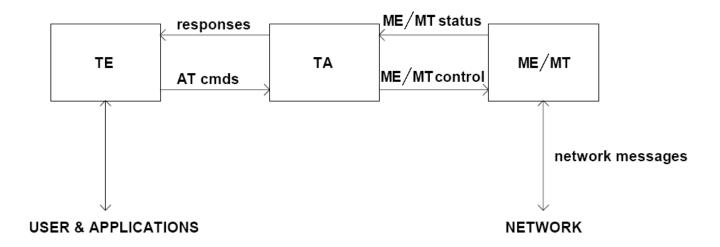
TELIT MODULEs physical implementation of this abstract architecture integrates the TA under the ME cover, and implements the TE as a separate entity.
