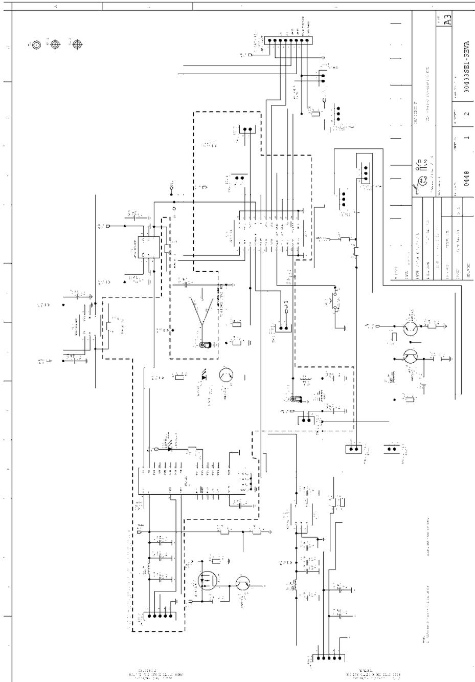
Figure 4-3 SL869-3DR EVK Board Schematic Diagram – Page 1 / 2
