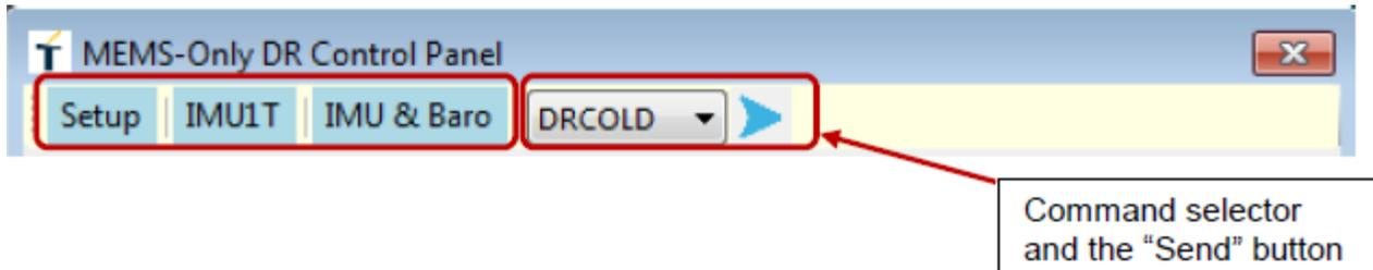
**Figure 7-0** Menu strip on MEMS-Only DR Control Panel
