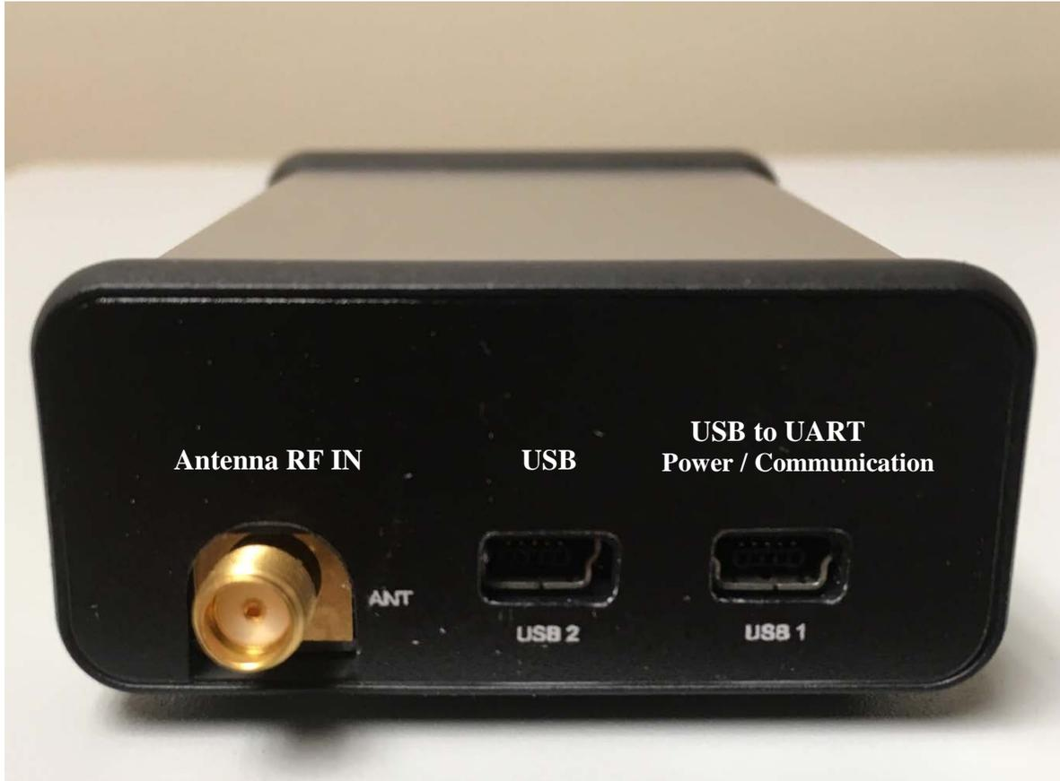
Figure 4-5 EVK Unit connections – rear panel
