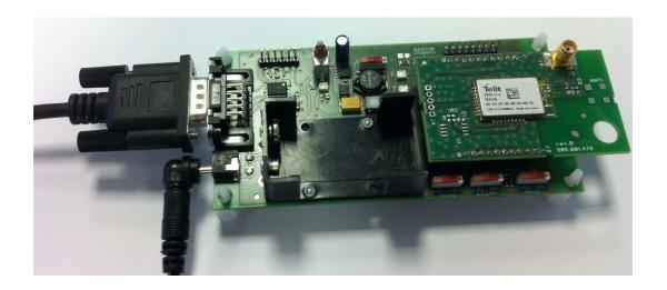
Step 3: Before switch on the EVK put PROG switch in ON position.
