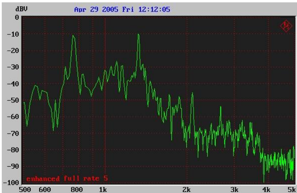
Figure 33. DTMF 5 dialing with Enhanced Full Rate compression type.
