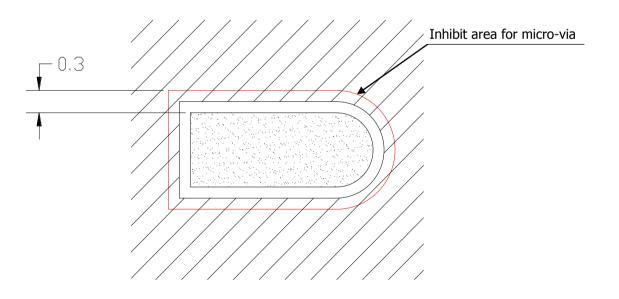
Holes in pad are allowed only for blind holes and not for through holes.
