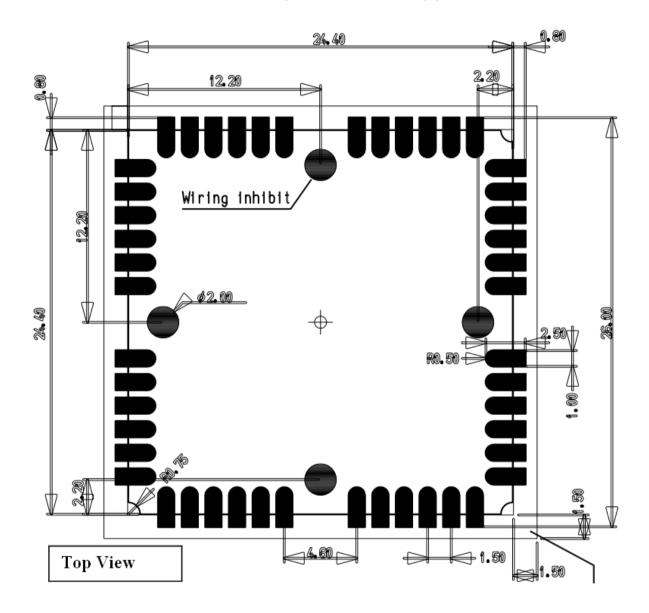
In order to easily rework the UL865-N3G is suggested to consider on the application a 1.5 mm placement inhibited area around the module.
