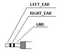
Or using the PL602 connector where the pin-out is the following:
