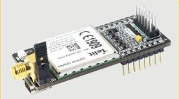
"t910 BoB" is a formative with a microBUS structure. It is an effective and easy solution for adding GSM/GPRS/3G/LTE solutions into your design. It features the Telit LE910-EU V2 or LE910-EUG module, a SMA connector for an antenna, a SIM CARD socket. t910 BoB communicates with thetarget board microcontroller via microBUS (Rx, Tx, Rx2, Tx2, RTS, CTS, Reset, GPIOs). The Audio Connector is compatible with Iphone, Samsung, HTC headsets. It has two LED diodes for power indicator and status.
